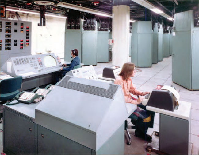
Historic photo of the MSDP control area on MCSB level 2. Control consoles and status displays are in the foreground while some of the 'digital racks' which housed the components for the MSDP computer are to the rear. Provided by Clint Esciklsen
